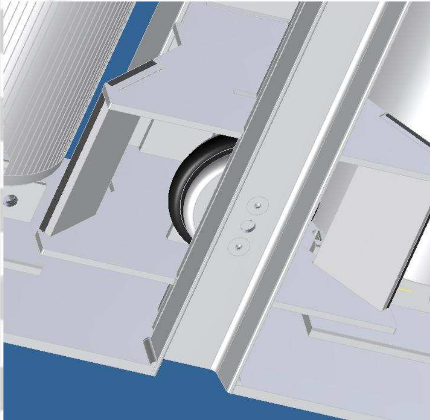
Figure 5 – Air Bag Bracket Assembly Mounting to C-Channel
