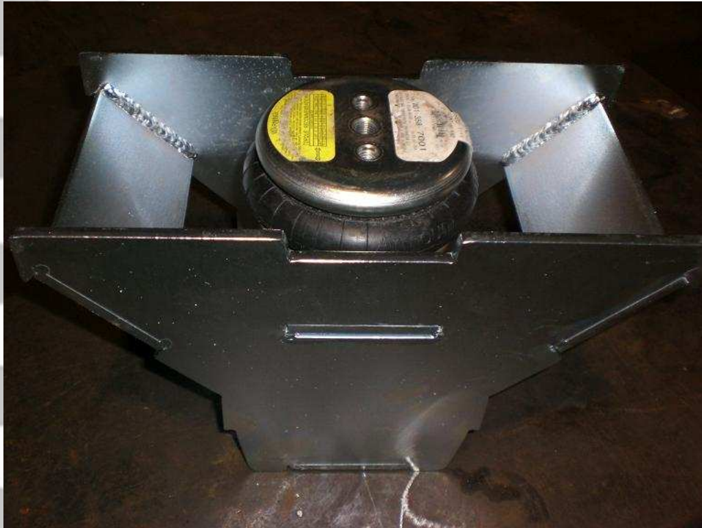
Figure 2 – Air Bag Installation
